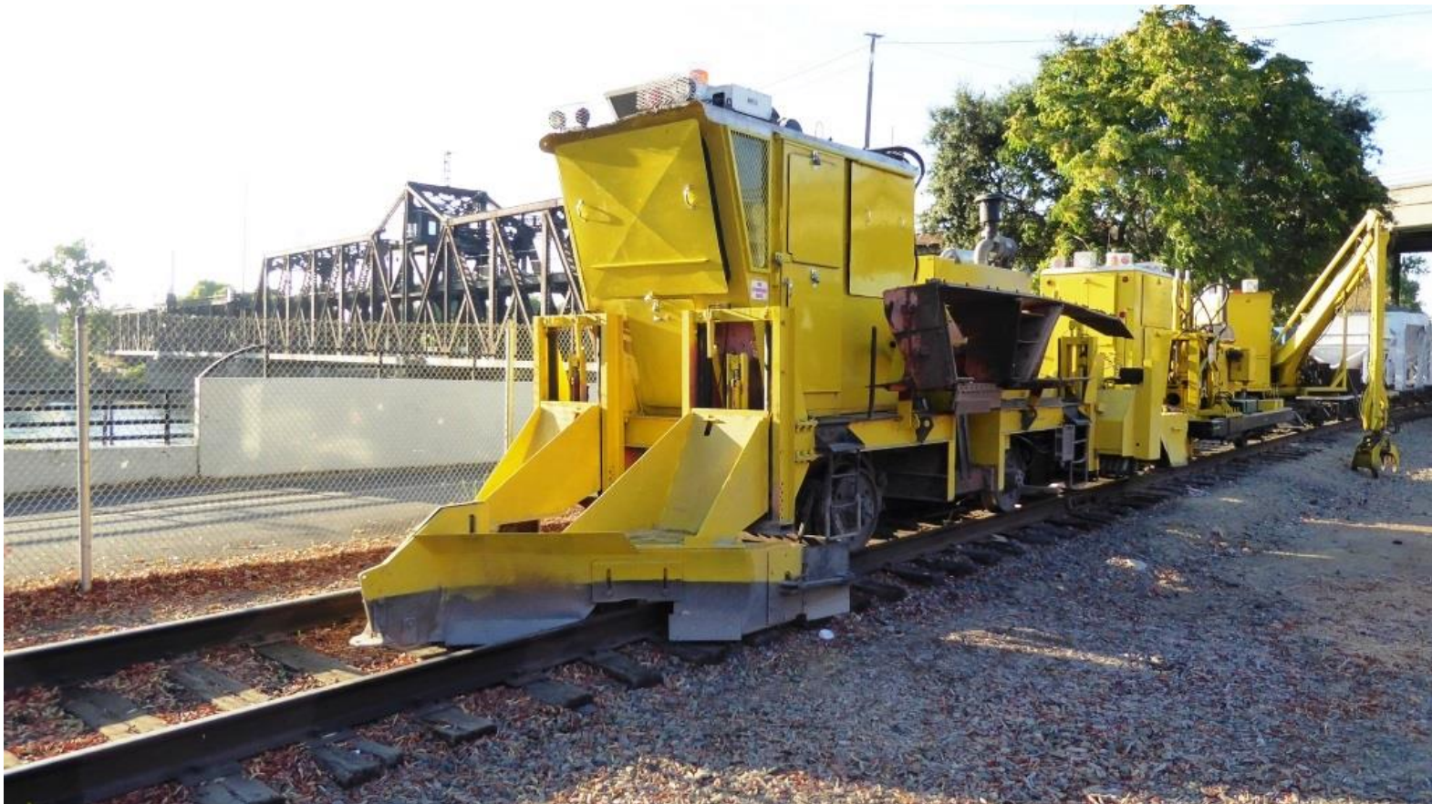
Raise shields! The ballast regulator fully protected from the whims of vandals
