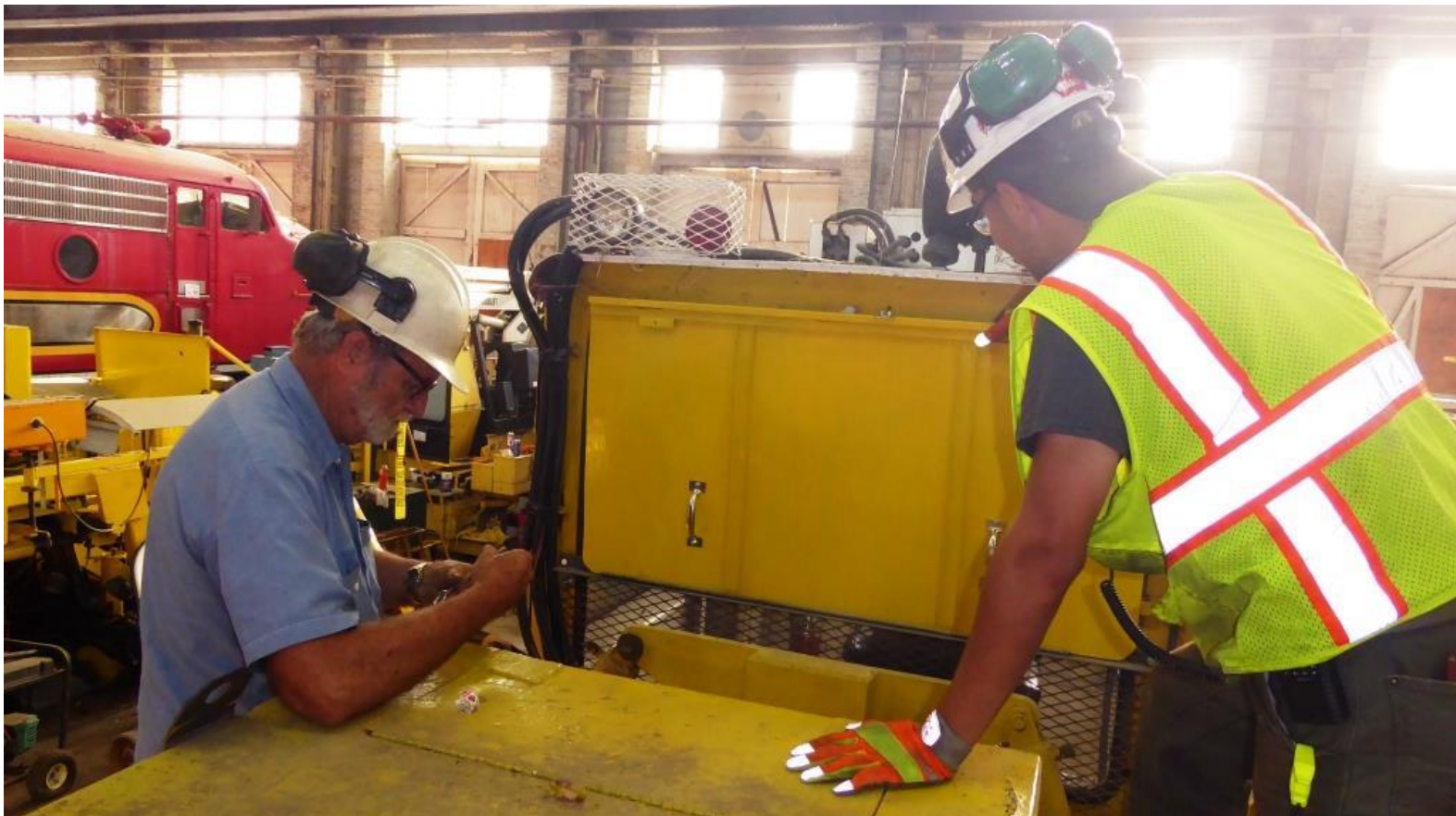
Alan and Kyle fit the final window shield into place on the regulator
