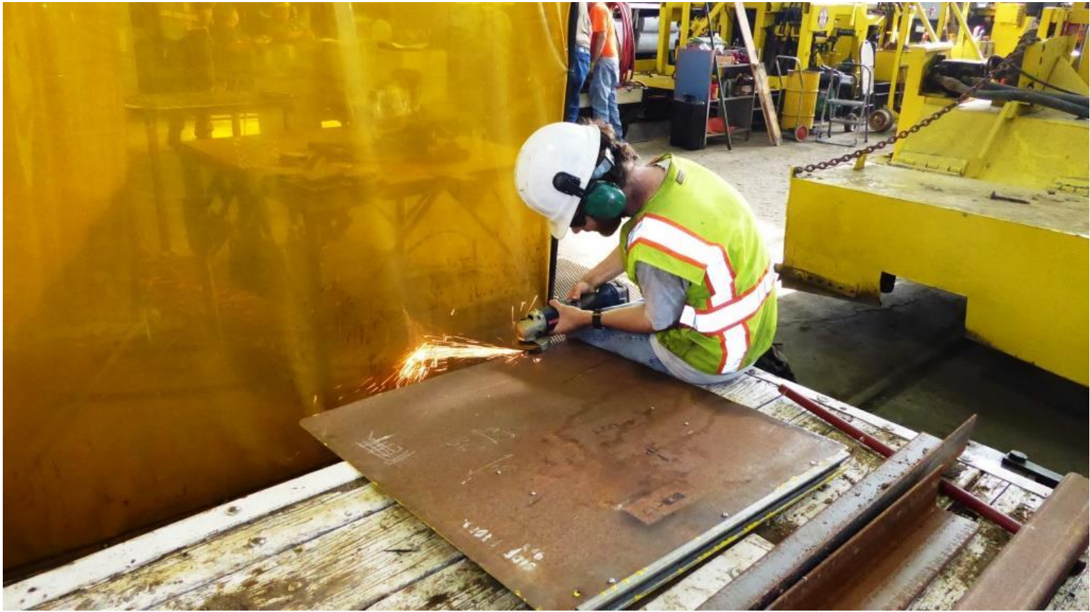
Matt grinds the edges of the final window shield for the ballast regulator
