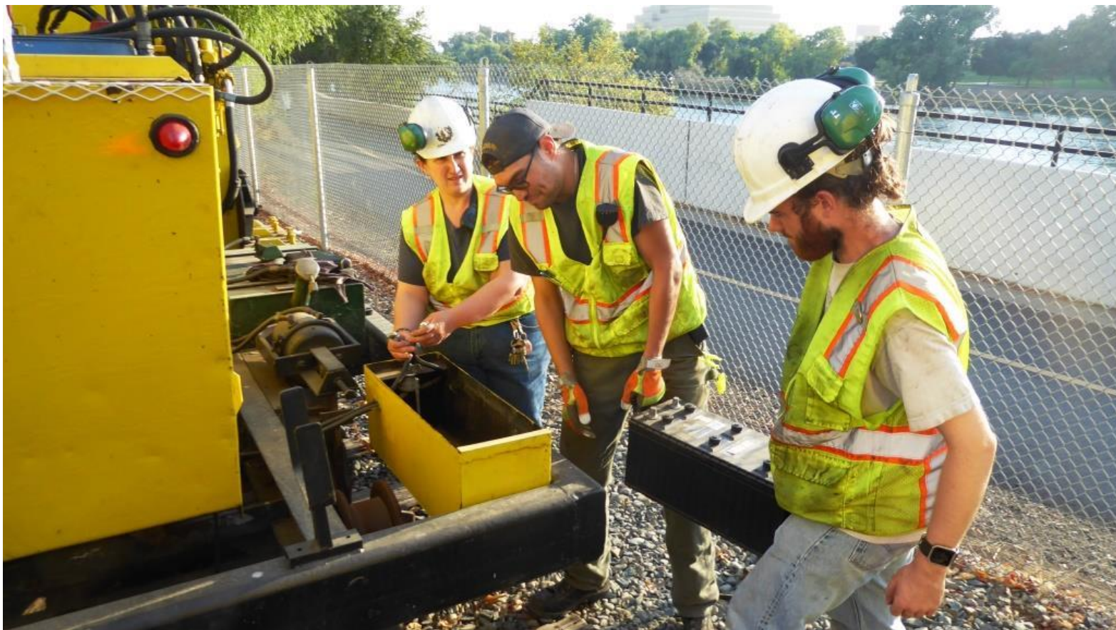
Over in Old Sac., Heather, Kyle, and Matt install the regenerated battery into the tie-shear
