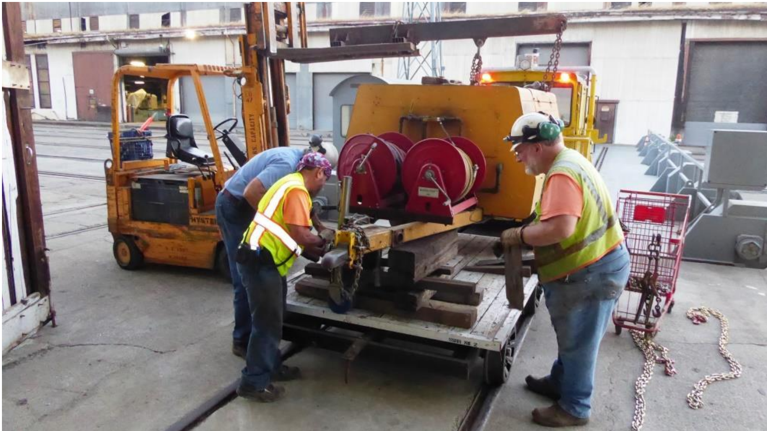
After loading the tire-mounted air-compressor on a flatcar, Alan, Joe, and Frank build cribbing under the hitch end for added support
